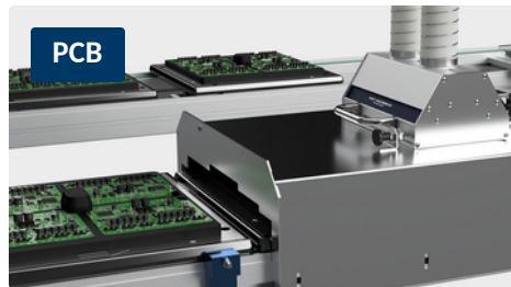
Cleaning of PCB Assemblies
