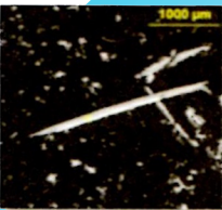
Particles from a screw fastening process
