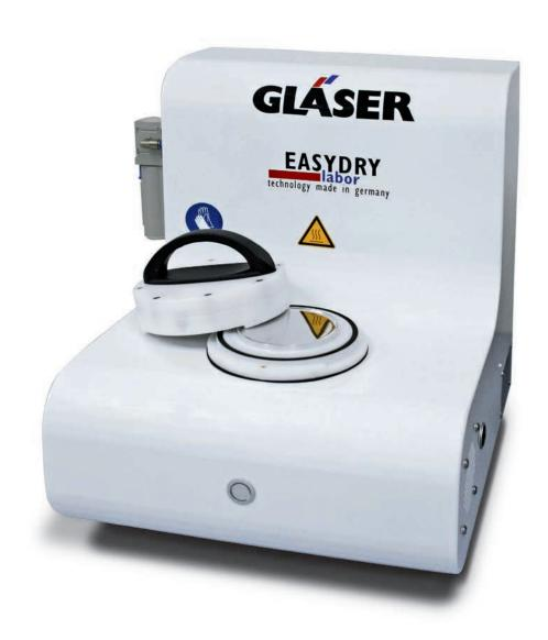
Device for drying analysis membranes for the determination of gravimetry of Technical Cleanliness of functionally relevant components in accordance with VDA 19.1 and ISO 16232. With significant time and place saving. Minimization of hazards when handling solvents in relation to conventional membrane preparation.
