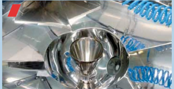
**The tank**, measuring 700 mm x 600 mm for components up to 15 kg. As on the ACM 17, combinable extraction options such as rinsing, spraying and flooding, incl. a 300 mm ultrasound tank. Optional funnel: small components subject to high demands can be tested more flexibly and quickly
