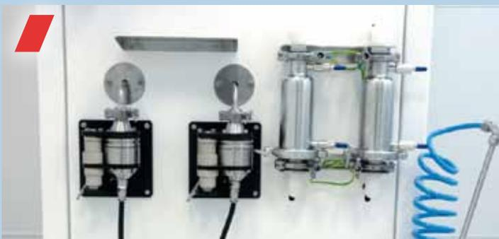
**Ergonomic membrane holder:** can be swung open. Incl. filter cascade for up to 3 analysis membranes. Optional second membrane holder for rinsing inside components
