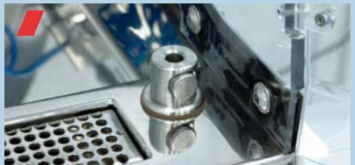
**Optional inside rinsing:** ideal possibility, unique on the market, of rinsing lines and components directly onto a second membrane holder
